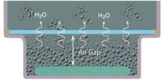
Traditionally, even though there are known limitations, the gravimetric test method, better known as the Wet Cup and Dry Cup versions of ASTM E-96 has been used to measure moisture through high transmitter barriers.
